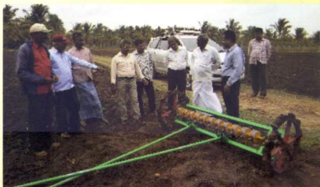
The new onion drum seeder being demonstrated in the farmer's field
