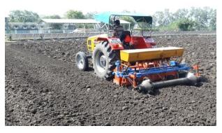
sowing at speed 3 km/h. Weight of the machine, with and without rotavator is 550 and 150 kg, respectively. Rolling type bed shaping system as power wheel is a special feature of this seeder. Due to rolling action of bed shaper attached in this machine, bigger size clods do not get exposed and a smooth bed is formed. The cost of the machine is Rs. 1,30,000/- (approx.).
