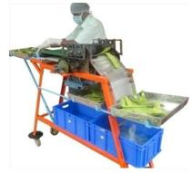
motorized and 100 kg/h (400 - 450 leaves/h) when operated manually. The saving in time and cost over conventional method is up to 70% and 50%, respectively. The aloin content in the extracted whole gel is within the acceptable limits. The cost of the equipment is Rs 60,000/- (approx.). The patent has been filed and equipment has been commercialised.
