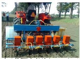
be varied by adjusting the clamps. The machine can save about 40-70% herbicide in comparison to blanket application. The initial cost of the applicator with inclined plate planter is Rs. 66,800/(approx.). The operating cost has been worked out as Rs 1350/ha. The same machine can be used as post-emergence herbicide/pesticide applicator after the removal of furrow openers and increasing the height of nozzles from the ground.
