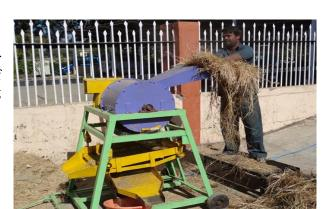
are 100 and 50 kg/h, respectively. The power requirement of the machine is 1.5 kW (2 hp), single phase electric motor. The overall dimensions of the machine (length, width and height) are  $1300 \times 1300 \times 1100$  mm. The weight of the machine is 150 kg and unit cost is Rs 45,000(approx.).
