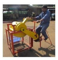
kernel breakage and dehusking capacity were 98%, 10% and 20 kg/h respectively. The unit costs Rs. 26,000/- (approx.).
