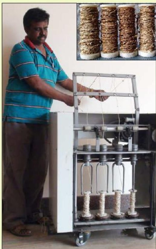
Fig. 8. Equipment for twisting and winding of splitted strands
