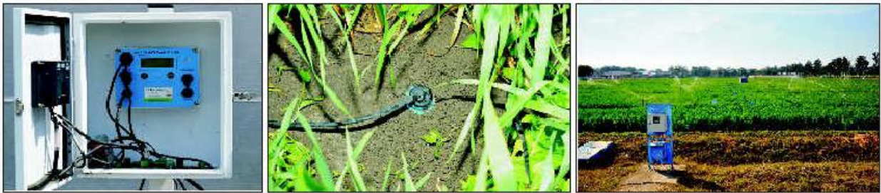
Fig. 15. Sensor installation and real time irrigation scheduling
