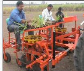
Fig. 26. Two row tractor operated sugarcane single bud settling planter
