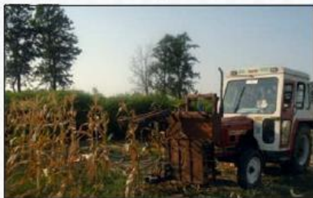
Fig. 16. Tractor front mounted hydraulic operated single row sorghum harvester
