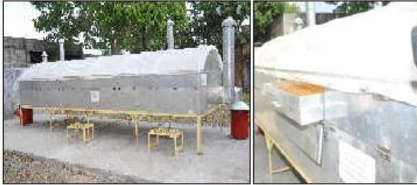
Fig. 25. The hybrid (solar biomass) hot air dryer
