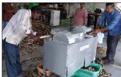
Fig. 17. Prototype model of double headed single bud cutting machine for sugarcane
