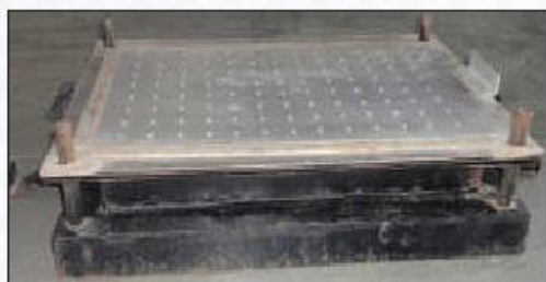
Fig. 23. Manually operated portray filling device
