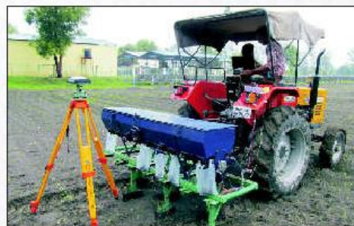
Fig. 2. GPS based variable rate granular fertilizer applicator system
