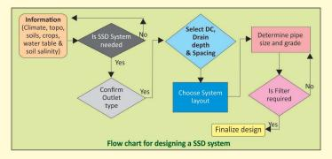
**Outlet:** Type and location of an outlet is the starting point in planning and designing a SSD system. Pumped or gravity outlet may be chosen as per the outfall condition. Pumped outlet is used in most canal/tubewell irrigation projects due to flat topography whereas gravity outlet is used in most lift irrigation projects.
