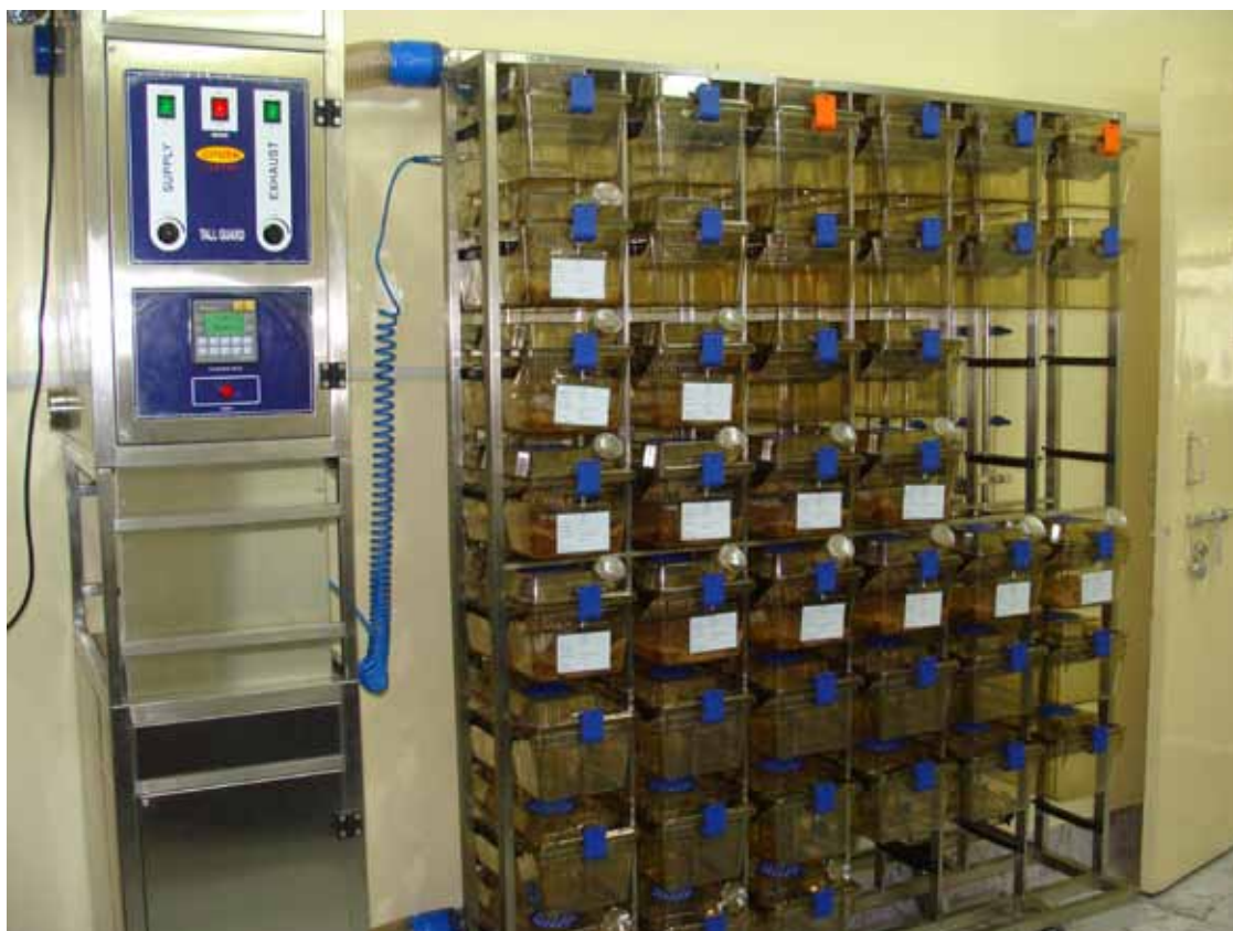
Fig. 69. Individual ventilated cages used for experimental intramammary infection in swiss albino mice.
