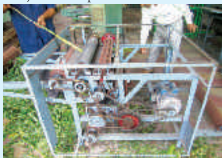
Figure QEI 13.1. Inside view of PALF fibre extractor
