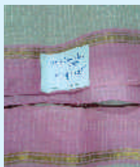
Fig QEI 8.7 Sizing of textile using mixture of Khoi & Dhaincha Gum
