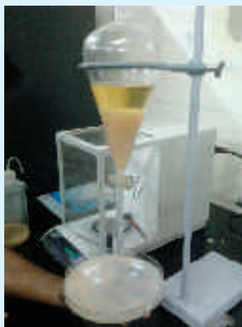
Figure QEI 8.1: Solvent extraction of dhaincha gum
