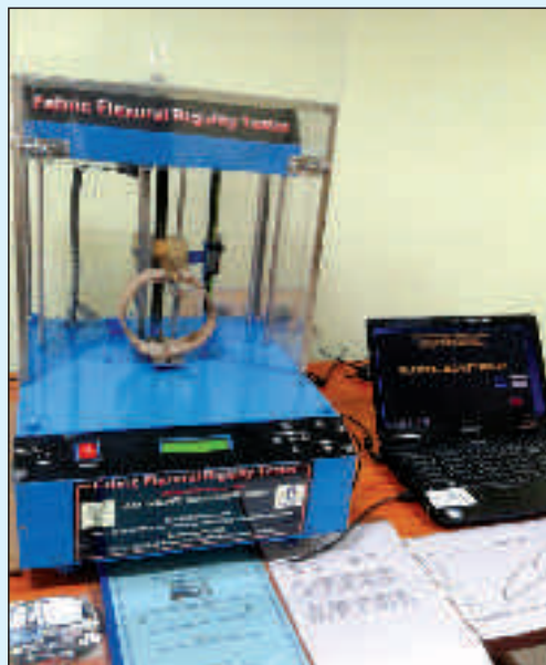
Figure IDP 19.1 - Flexural rigidity tester with preprocessing, storing & printing devices
