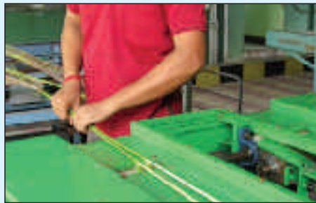
Figure TOT 9.2 : Ribbon/bark peeling through newly developed NIRJAFT power ribboner
