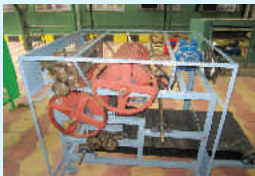
Figure QEI 12.1. Inside view of banana fibre extractor
