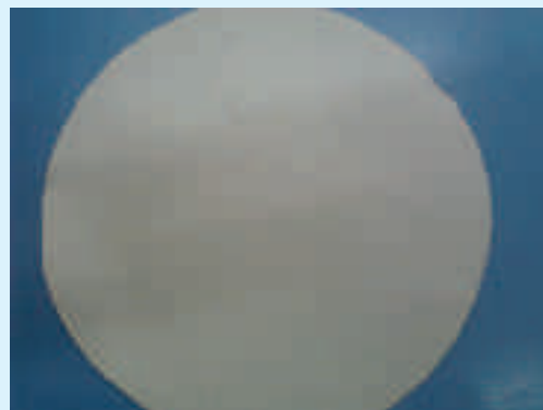
Figure QEI 8.4. Paper sample made up of jute fibre using dhaincha gum
