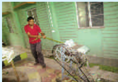
Figure TOT 9.5 : Ribbon/bark peeling through CRIJAF Bast Fibre Extractor
