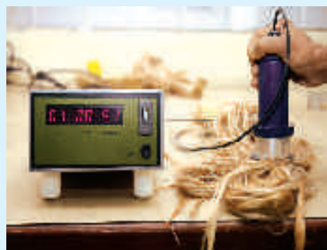
Figure QEI 16.2. Laboratory type Electronic Colour and Lustre
