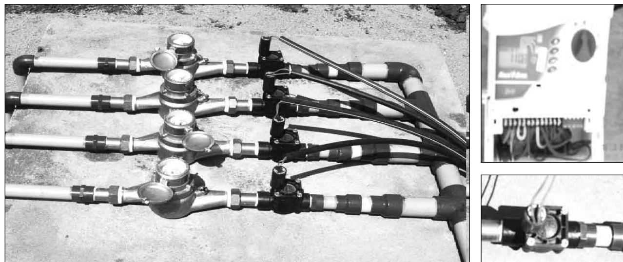
Fig. 1. The automatic drip irrigation scheduling hybrid stations controller (E-6) and solenoid valves
