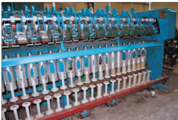
Automated flyer spinning machine for jute-coconut fibre
