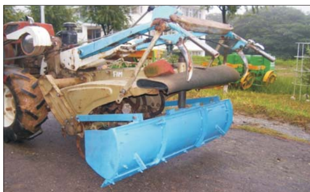
Power tiller-operated bench terracer-cum-leveller
