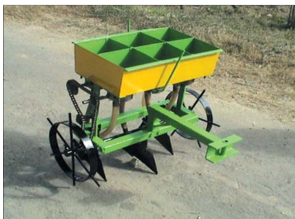
Power tiller-operated zero-till drill
