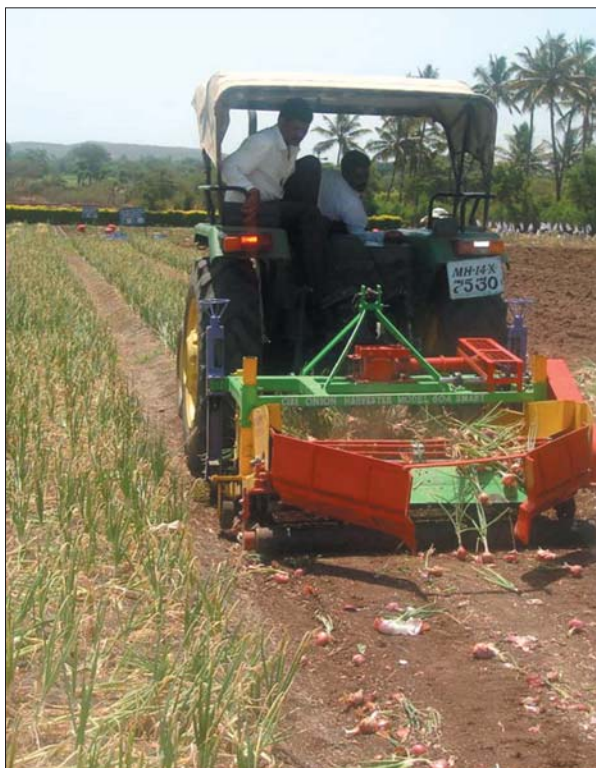
CAD model of tractor-operated rear-mounted onion harvester (left) and onion harvester under evaluation (right)
