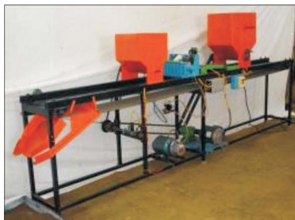
Needle type tray seeder for vegetable nursery production
