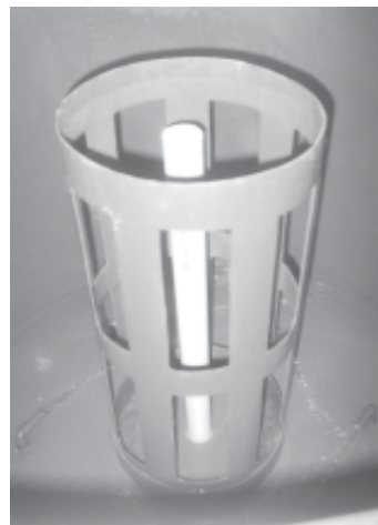
FRP hatching pool inner chamber
