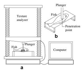
Fig. 1. (a) Experimental set up of texture study of iced storage of fish; (b) showing the selected sampling area.
