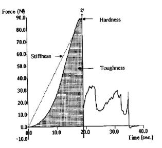
Fig. 2. Typical force-time deformation curves during compression/ penetration for *Rohu* fish.
