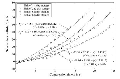
Fig. 3. Representation of modified Maxwell model for force-time relationship for fish skin hardness stored in ice.
