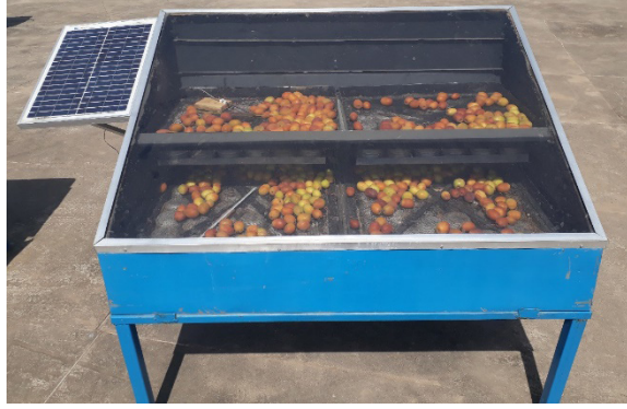
Fig. 2: Indian jujube in PVT hybrid forced convection solar dryer installed at CAZRI solar yard
