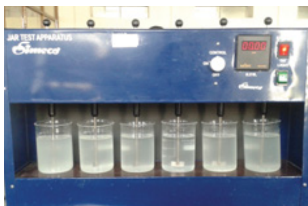
Fig. 51. Flocculation evaluation with Jar test apparatus
