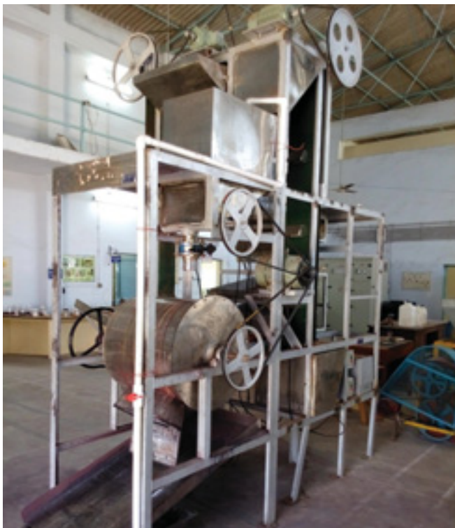
Fig. 36. Integrated small scale lac processing unit
