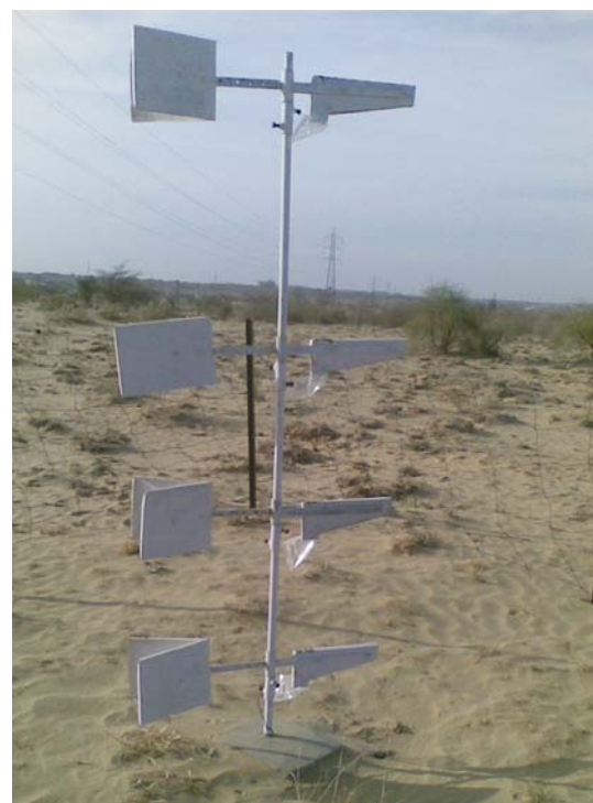
Figure 2. The new wind-erosion sampler installed at the field site of Jaisalmer station of CAZRI located in the Indian Thar Desert.
