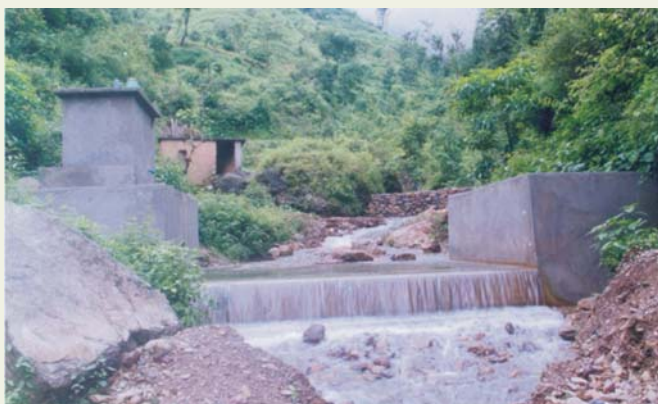
Monitoring station for appraisal of soil erosion by water in lower mid-Himalayas
