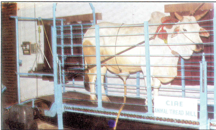
Fig. 4 : Bullock on the tread mill with single harnessing system
