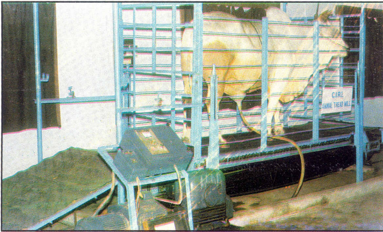
Fig. 5 : View of variable speed motor and reduction unit connected with the tread mill
