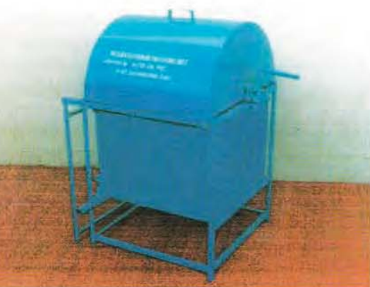
Integrated turmeric processing unit
