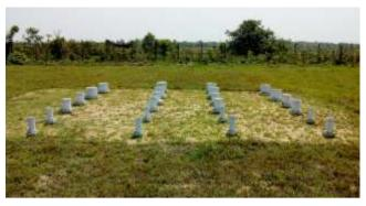
Mini pan-evaporimeters (GI and PVC) of different sizes installed at ICAR-IIWM research farm, Mendhasal
