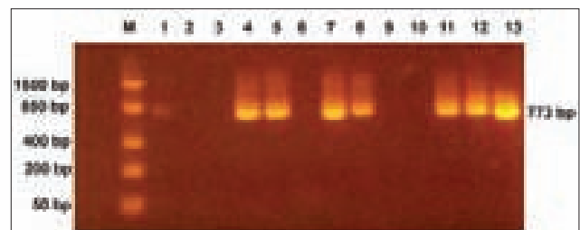
Amplification of bla TEM gene ( Lane 1,4,5,7,8, 11,12: Test positive; Lane 2,3,6,9,10: Test negative; Lane 13: Positive control; Lane M: Fast ruler low range DNA ladder)
