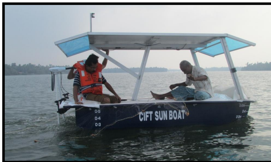
Fig.1. Solar powered inland fishing boat designed and constructed by ICAR-CIFT in gill net operation
