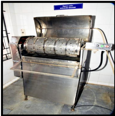
Fig. .6 Fish de-scaling machine with variable drum speed
