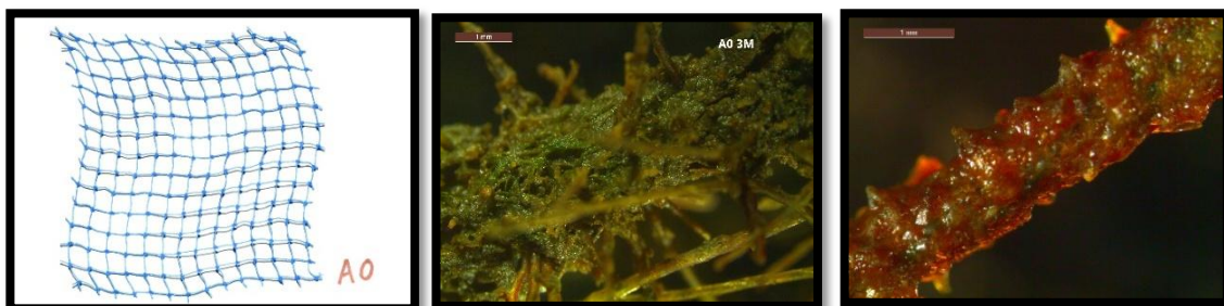
Fig 2. A) PE cage net b) PE cagenet after 3 months c) PE cagenet treated with PANI+nano CuO after three months exposure in the estuary.
