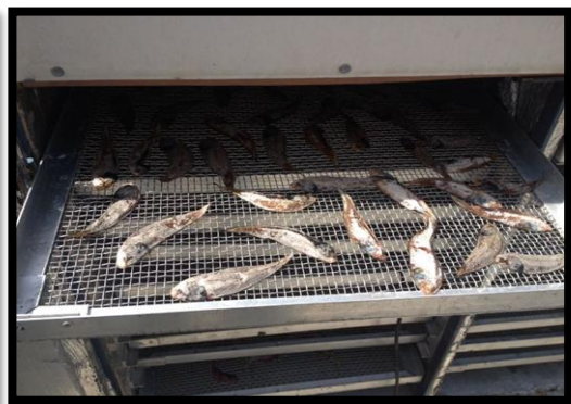
Fig.5. CIFT Solar-Cabinet Dryer with Electrical back-up
