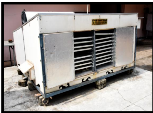
Fig.5. CIFT Solar-Cabinet Dryer with Electrical back-up
