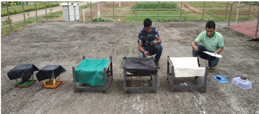
Fig. 2: Arrangement of different materials under natural conditions to record light intensity, temperature & relative humidity
