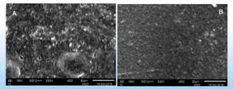
SEM micrographs of surface-section from sodium alginate films incorporated with GTE. A: pure sodium alginate films; B: sodium alginate films incorporated with 1% GTE
