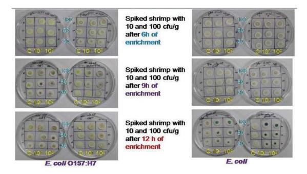
Detection of E. coli O157:H7 and E. coli from spiked shrimp by using paper strip
