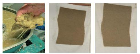
Water hyacinth pulp, non-absorbant fiber layer and absorbant fiber layer
