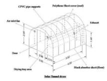
SS Schematic diagram of Solar tunnel dryer
