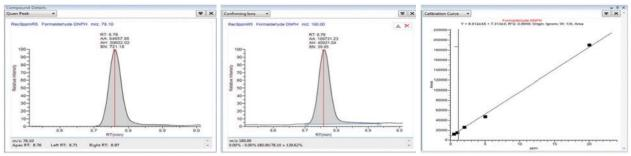
Quantifier transition Quantifier transition Matrix based calibration 0.5 to 20 ppm; R2: 0.9949
