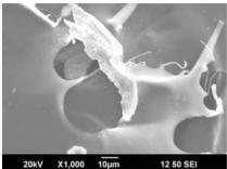
Scanning electron microscope (SEM) images of Chi-Ag-NPs
