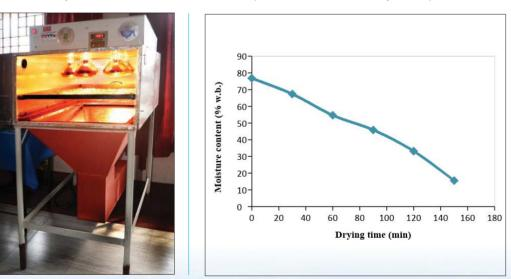
Prototype of hot air assisted infrared dryer and drying curve for shrimps
