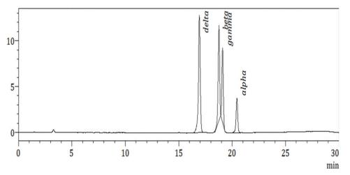
Chromatographic separation and quantification of isomers of tocopherols
