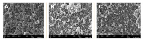
A) SEM of spray dried SFB) SEM of encapsulated SF with maltodextrinC) SEM of encapsulated SF with maltodextrin and sodium casienate
