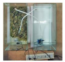
Re-circulatory system to determine bioremediation potential
