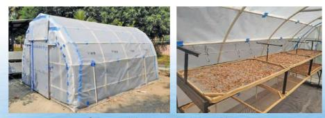
Solar tunnel dryer under loaded conditions
