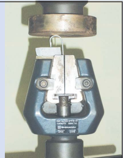
Experimental setup showing sharpness test using Universal Testing Machine
