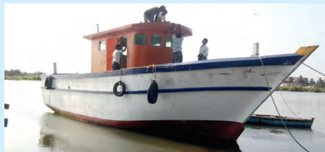
13.7 m L OA FRP Tuna fishing boat for Andaman and Nicobar Islands ready for stability test at Cuddalore
