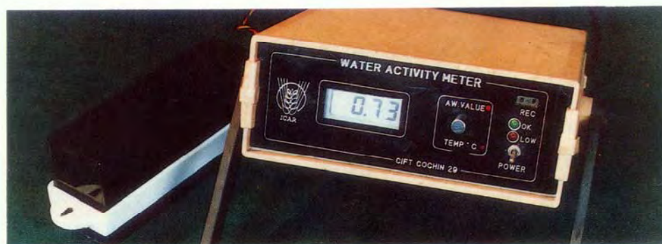
The Water Activity Meter developed at the Institute for measuring the a_w value in food materials
