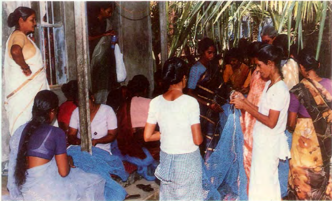
'Women in Agriculture' Day - women being trained in fabrication of trawl cod ends and webbings for polypropylene trammel nets
