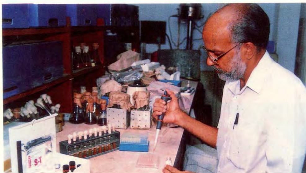
ELISA (Enzyme - Linked Immunosorbent Assay) technique for rapid detection of Salmonella in fishery products
