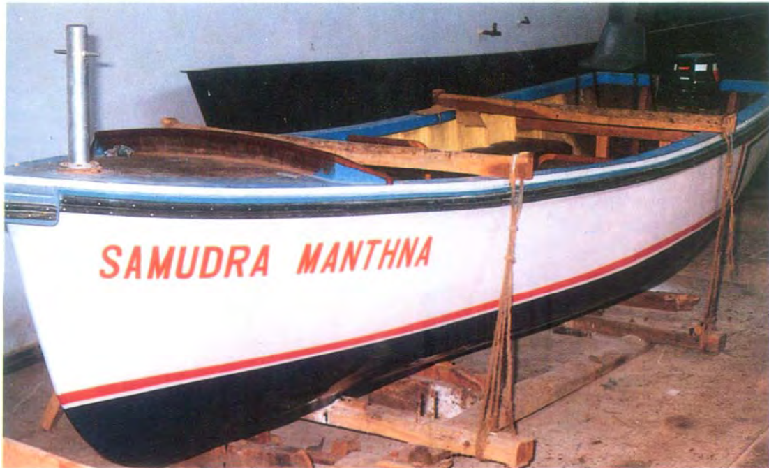
A 7.64 m. fibreglass boat designed and developed at CIFT for pole and line fishing around Lakshadweep Islands.
