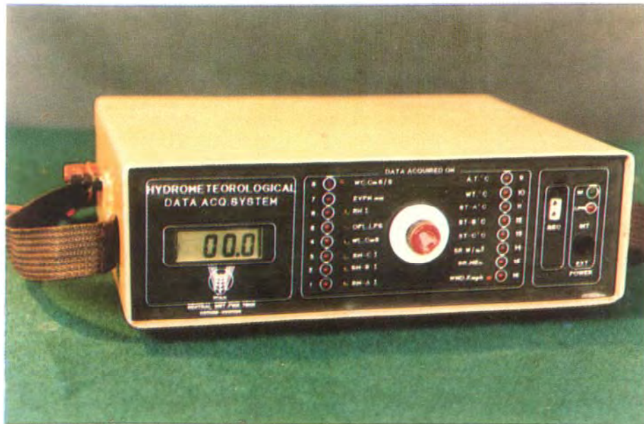
Hydrometeorological data acquisition system for acquiring 16 channel data from soil, water and air
