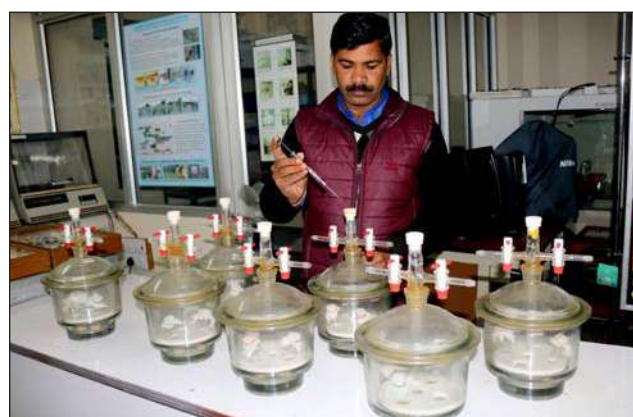
Bioassay on phosphine with modified desiccator
