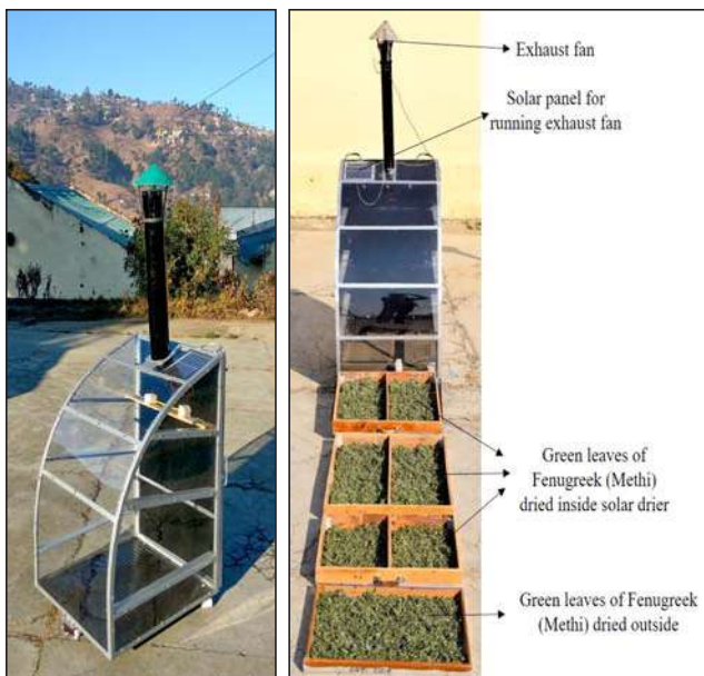
Portable plastic solar cabinet dryer for hilly region
