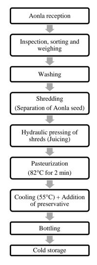
Figure 2. Process Flow Chart for Aonla Juice Preparation
