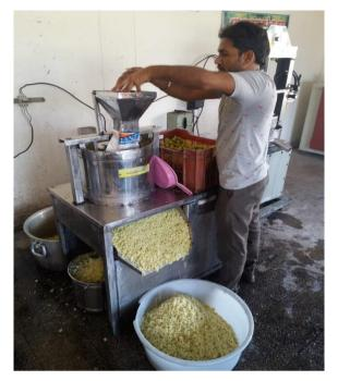
Figure 3. Aonla Shredding in Operation Performed by the Entrepreneur
