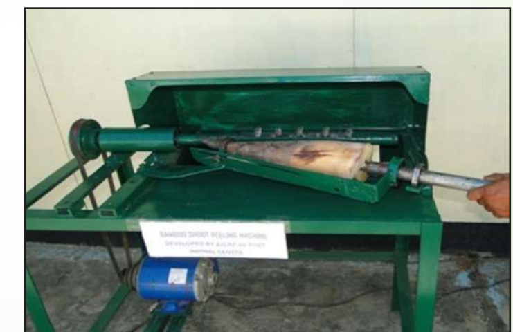
Figure 6: Bamboo shoot peeling machine
