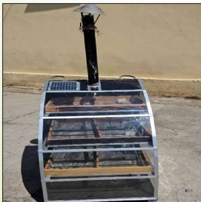
Figure 8: Solar Cabinet Dryer for operation hilly region
