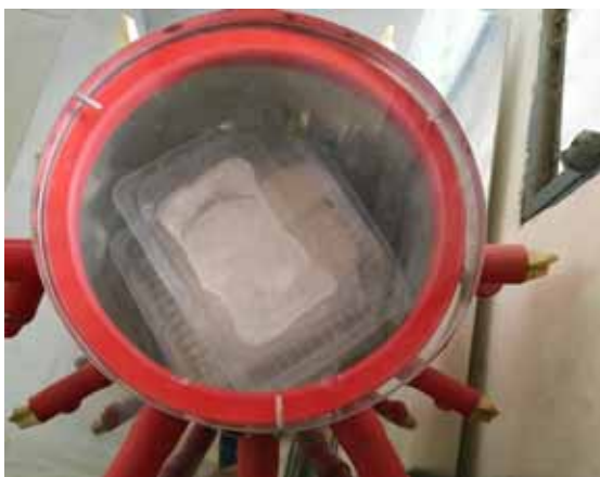
Freeze drying of sample using lyophilizer
