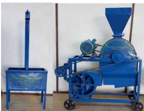
Hand and power operated Water chestnut decorticator
