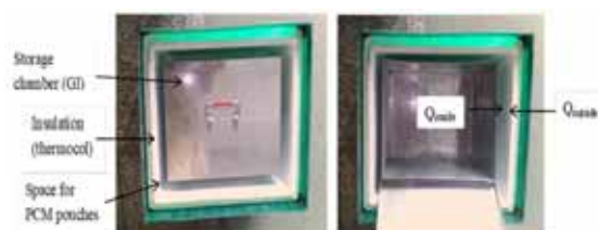
Prototype of PCM-based cool chamber
