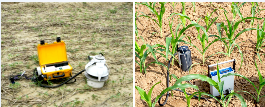
Fig. 3. Collection of CO 2 samples from field using the Infra-red analyzer and soil respiration chamber method
