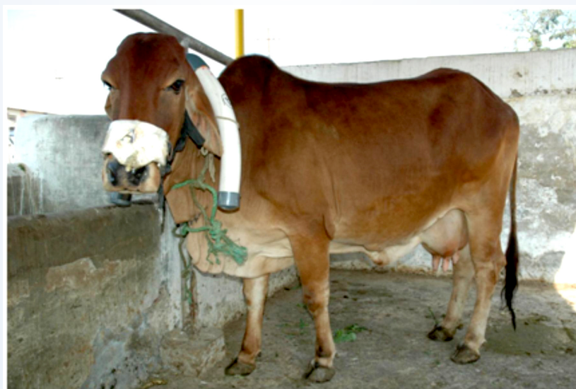
Fig. 2. Neck halter and capillary tube system on nostril area for measuring SF 6
