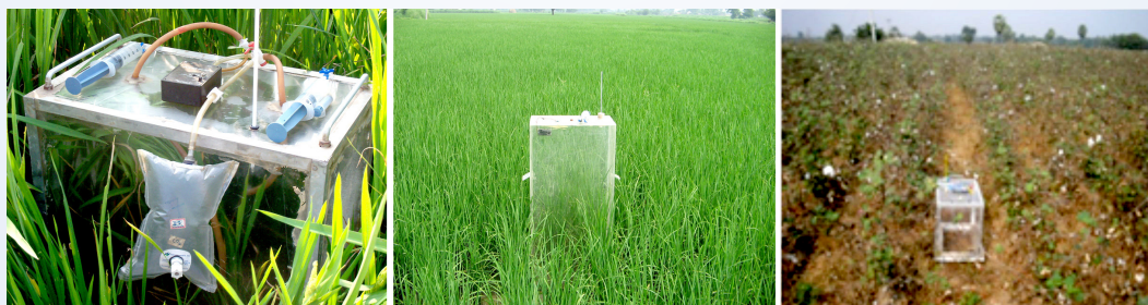
Fig. 2. Collection of GHGs samples from field using the closed-chamber method
