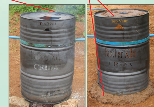
Field operational process in biochar production
