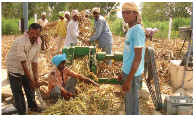
Crushing operation at decentralized cluster unit
