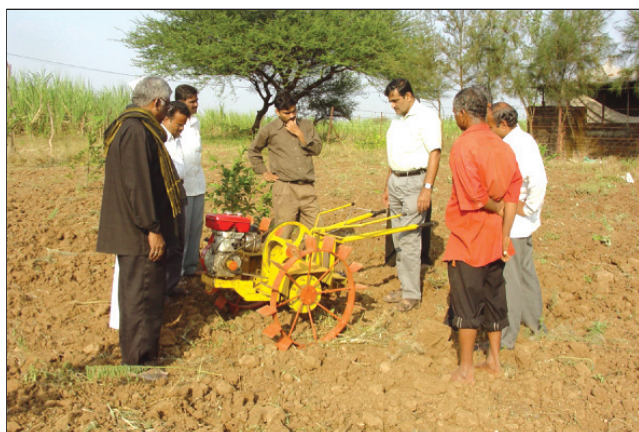
Multipurpose self propelled (5 hp) machine for dryland field operations
