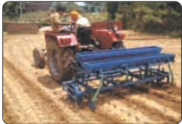
Sowing of greengram with zero till drill (left) at SK Nagar, Gujarat, and maize with maize planter at Rakh Dhiansar, Jammu & Kashmir
