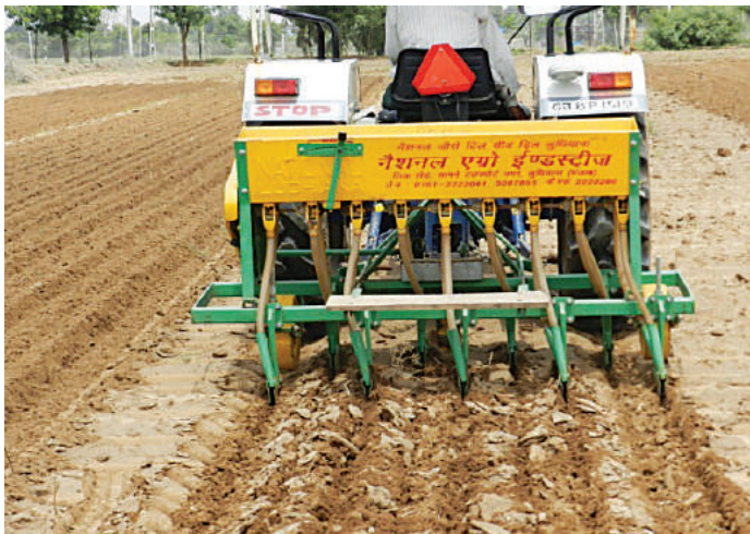
Sowing of greengram with zero till drill (Kalimati/Dholiya, Banaskantha district)
