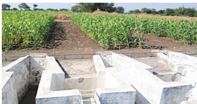
Runoff plots with multislot measuring devices in Sorghum and Sunflower
