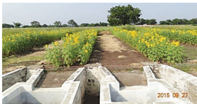
Runoff plots with multislot measuring devices in Sorghum and Sunflower
