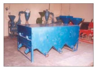
Rotary screen grader for raw pulses and separation of finished products
