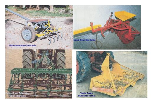
**Bed-furrow formers**: Though animal drawn bed –furrow formers are available, their efficiency is very less. The tractor drawn be-furrow former is capable of forming alternate beds and channels. It saves 90 % of labour. These beds are suitable for planting crops like sorhum maize, cotton. This sbed and furrow system is ideal for efficient irrigation management.
