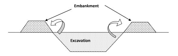
Fig 3.4 Excavation of pit and embankment of the dug out soil
