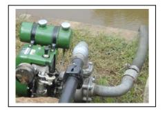
Plate-3 Portable Diesel Pumpset of 1.5 Hp
