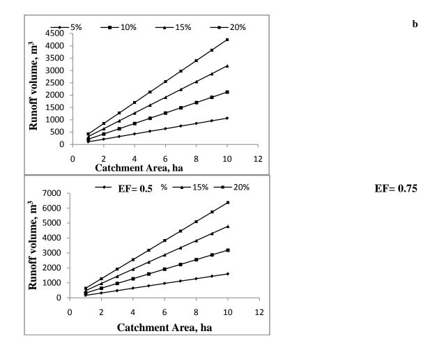
Fig 2(b). Expected runoff volume at design seasonal rainfall 425mm (67% probability) for varying runoff coefficients, efficiency factor (EF) and catchment area.
