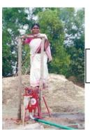
Fig-2 Pedal operated reciprocating pump
