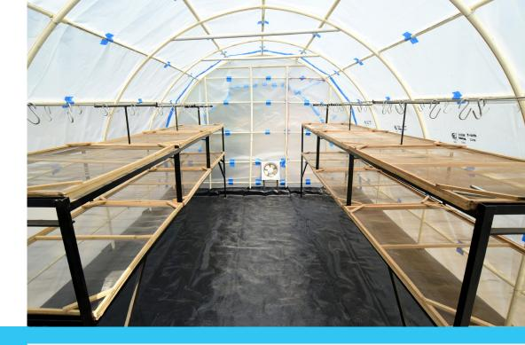
ICAR-CIFT developed a low cost, energy efficient solar tunnel dryer for bulk drying of fish and fishery products. This dryer can be used by fishermen or small-scale fish processing units for bulk drying during seasonal higher catch/excess landing of fish. The capacity of the solar tunnel dryer is 50 kg with the floor area of 12 m². The materials of construction are UV stabilized transparent polythene sheet for roof cover, black absorber sheet for floor, supporting frames of CPVC and GI rod.
