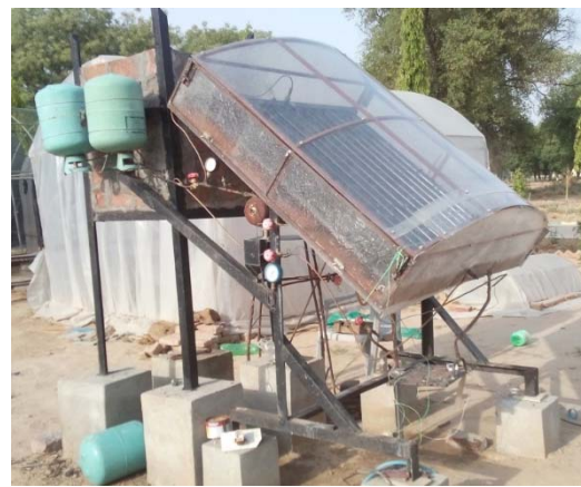
solar energy based vapor adsorption cooling system
