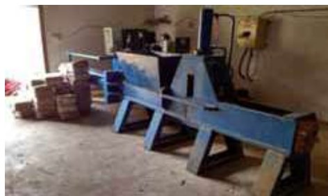
Fig. 5. Feed block making machine (after mixing with ingredients) (Source: IARI, New Delhi)
