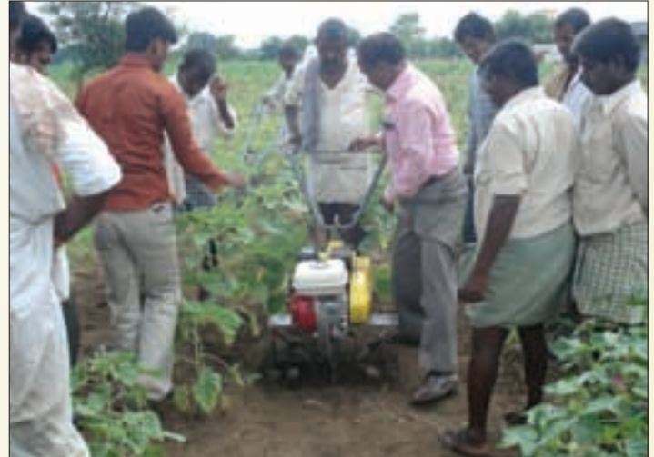
Demonstration of the operation of 5.5 HP power weeder in cotton
