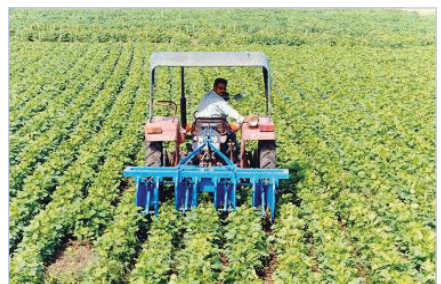
Fig 25.6 Rotary power weeder (courtesy: NRC soyabean)
