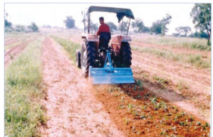
Fig 25.2 Residue incorporation with rotavator
