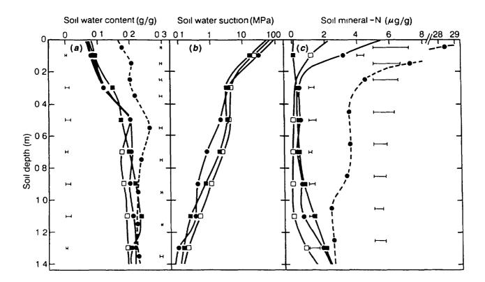
FIG 4 Soil profiles of (a) water content (b) water suction and (c) mineral-N concentration, sampled at maturity (solid lines) of wheat crops following canola ( $\bullet$ ), Indian mustard ( $\Box$ ) and wheat ( $\blacksquare$ ) Water content and mineral N at sowing (dashed line) for the wheat following wheat are also presented. Horizontal bars represent standard errors of means [9]
