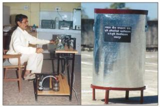
Foot operated vacuum packaging machine (left) and double walled thermocol filled GI container (right)
