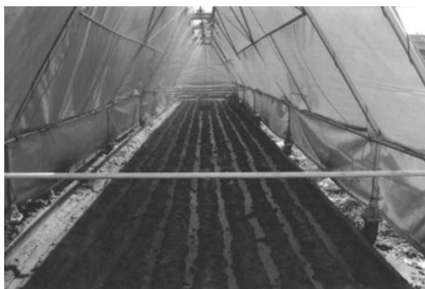
Figure 4 Simulator with furrows down the slope at 30 cm spacing.
