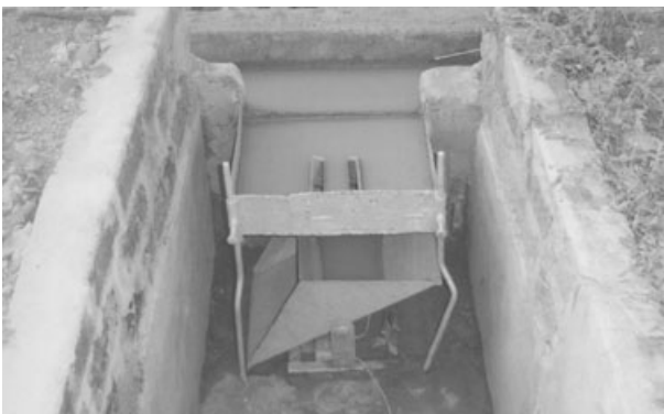
Figure 3 Tipping bucket assembly at the outlet of the runoff plot.
