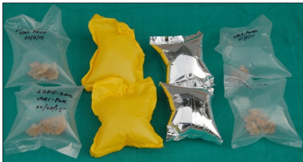
Fig. 1. Gum karaya samples packed in LDPE, HDPE, ACP and PP film with nitrogen filling
