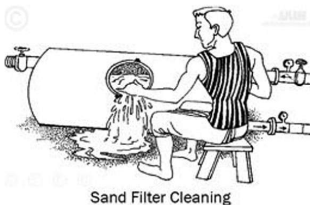
Fig. 25. Cleaning of the sand filter by stirring the sand (From Jain Irrigation systems)
