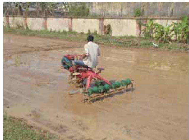
Fig 44. Self-propelled drum seeder with hyperboloid drum
