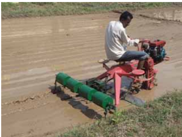
Fig 43. Self-propelled drum seeder with cylindrical drum
