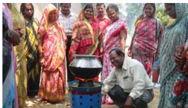
Demonstration of CRRRI rice-husk stove for effective use of rice by-products
