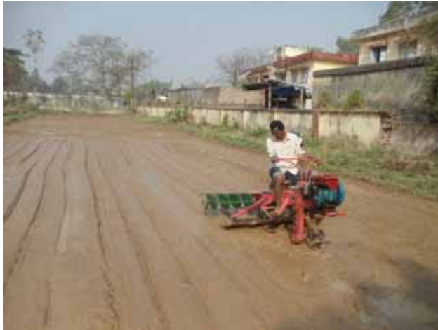
Fig 42. Self propelled drum seeder with cup type feed mechanism
