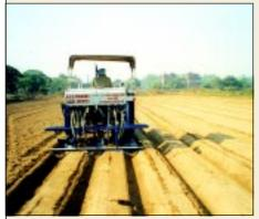
Wheat raised-bed planter. Its cost of operation with 45-hp tractor for fresh beds is estimated at Rs 200/hr. With this, wheat yields obtained were 4.48 tonnes/ha, compared to 4.08 tonnes/ha of flat sowing
