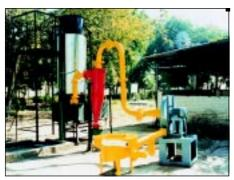
**Groundnut-shells-based Open-core Gasifier.** The fuel used for the system is dry groundnut-shells and groundnut-shell briquettes. In the system, every 4 kg of groundnut-shells replaced 1 litre of light diesel oil
