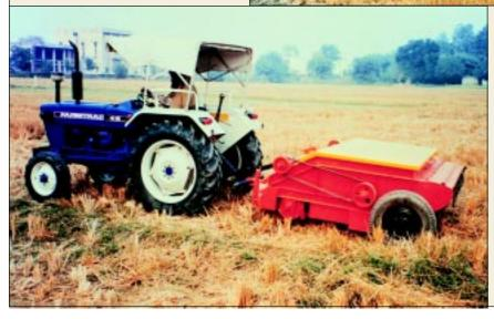
**Tractor-operated straw-chopper-cum-spreader**. For rice-straw management, a tractor-operated, straw-chopping machine has been developed. The machine chops straws of 5-cm length and spreads it in the field. Its capacity is 4 ha/day
