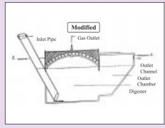
Line diagrams of conventional (left) and modified (right) Janta Biogas plant
