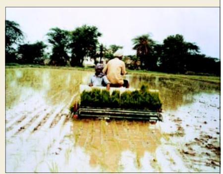
Modified PAU self-propelled rice transplanter. The estimated cost of the machine is Rs 70,000 as against Rs 120,000 of the imported unit
