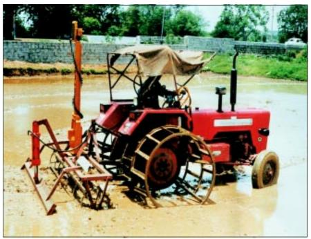
ANGRAU tractor-operated laser-controlled wetland leveller. This has given encouraging results for precision levelling in wet conditions. Its field capacity is 1.8–2.5 ha/day at 3–4 km/hr speed
