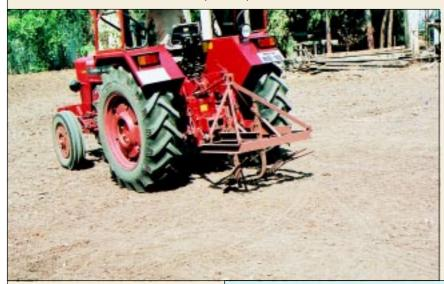
**Tractor-mounted turmeric digger**. It could dig turmeric bulbs from 12-cm depth with 4% bulb damage
