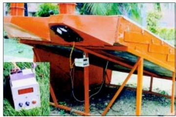
Electronic temperature controller fixed with a natural convection solar dryer. This is now commercially available.
