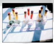
Higher HCN content in leaves of bamboo restricts its feeding to livestock. Sun-drying, boiling and oven-drying of bamboo greatly reduces the HCN content
