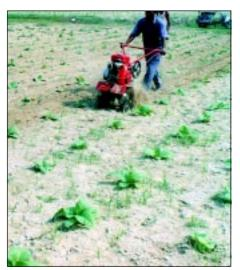
Light weight power-weeder for interculture. It is found suitable for weeding with 40-cm rotavator and rotary wheel. There is a net saving of Rs 1,070/ha with this, compared to traditional method of interculture
