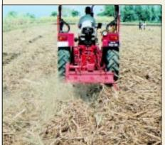
**Tractor-mounted sugarcane trash-shedder**. Its soil-mixing blades dig soil from the sides of the ridges and mix it with chopped trash. Due to its soil digging, fibrous roots of stubbles could be removed; which is useful for the ratoon-crop
