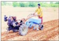
Power tiller-drawn seed-cum-fertilizer drill/ planter was engineered for sowing blackgram, greengram, sorghum, groundnut, maize and castor. It has an area coverage of 0.25–0.3 ha/hour
