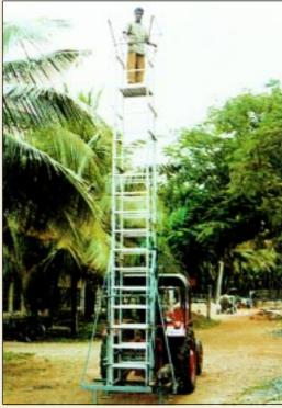
Tractor-mounted hydraulically-opeated hoist for harvesting mango, guava, sapota and coconut. It is safe and stable in operation, and easy to transport, and its cost of operation is Rs 336/hr
